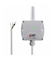
The device measures the temperature from the built-in sensor with the possibility of installation directly into the measured space thanks to IP65 protection and DC voltage in range -30 to +30 V. By measuring the DC voltage, it is possible to remotely monitor, for example, the status of power batteries or, in general, the power status of the monitored technology. The input can also be used to connect sensors of various quantities with a standard output, eg 0-10 V.
