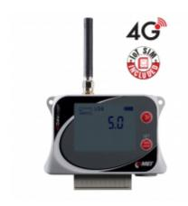
4G datalogger is designed to record 3 voltage inputs and 1 binary input. In case of exceeded set limits, SMS and JSON messages can be sent via 4G data connection. Measured values can be sent to the internet storage <a href="COMET Cloud">COMET Cloud</a>, which is a complete monitoring, alarm and analysis system.
