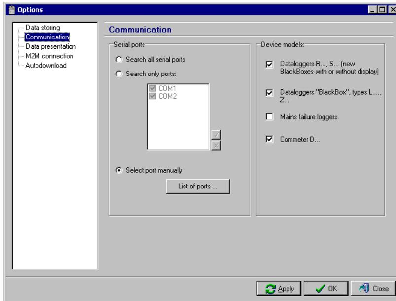
Select the item *Select port manually* and press the button *List of ports....* The window *List of communication ports* will be displayed. In this window, press the button *Add port*. The window *Add communication port* will be displayed.
