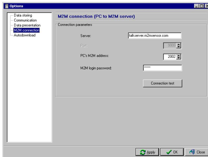
The items *Server* and *Port* are already pre-filled, don't change it gratuitously! Fill the items *PC's M2M address* and *M2M login password* with data listed in the card which was delivered with the modem. Confirm these settings with pressing *Apply* button.
