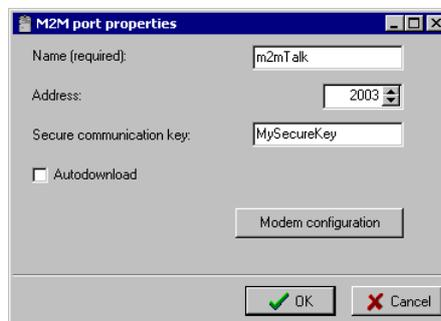
The window *M2M port properties* will be displayed. Set the connection parameters for the modem here. The item *Name* is intended for user's description of connection, choose your own name. Fill the item *Address* with data listed in the card which was delivered with the modem. If you want to prevent unauthorized access to your modem (recorder), you will have to fill the item *Secure*
