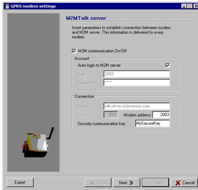
In this window, enter *Security communication key* according to setting in the window *M2M port properties*. If you require the modem's login on the server automatically after its switching on (so that GPRS communication can be available), you will have to tick off the field *Auto login to M2M server*. Don't change other parameters in this window gratuitously, it can cause problem with communication!
