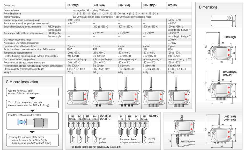
\*\*\* the accuracy of the device without probe in the range of -200 to +100 °C is ±0,2 °C (in the temperature range of +100 to +260 °C is accuracy ±0,2 % of measured value) \*\*\*\* for correct temperature measurement using thermocouples, it is necessary that there are no rapid temperature changes around the device
